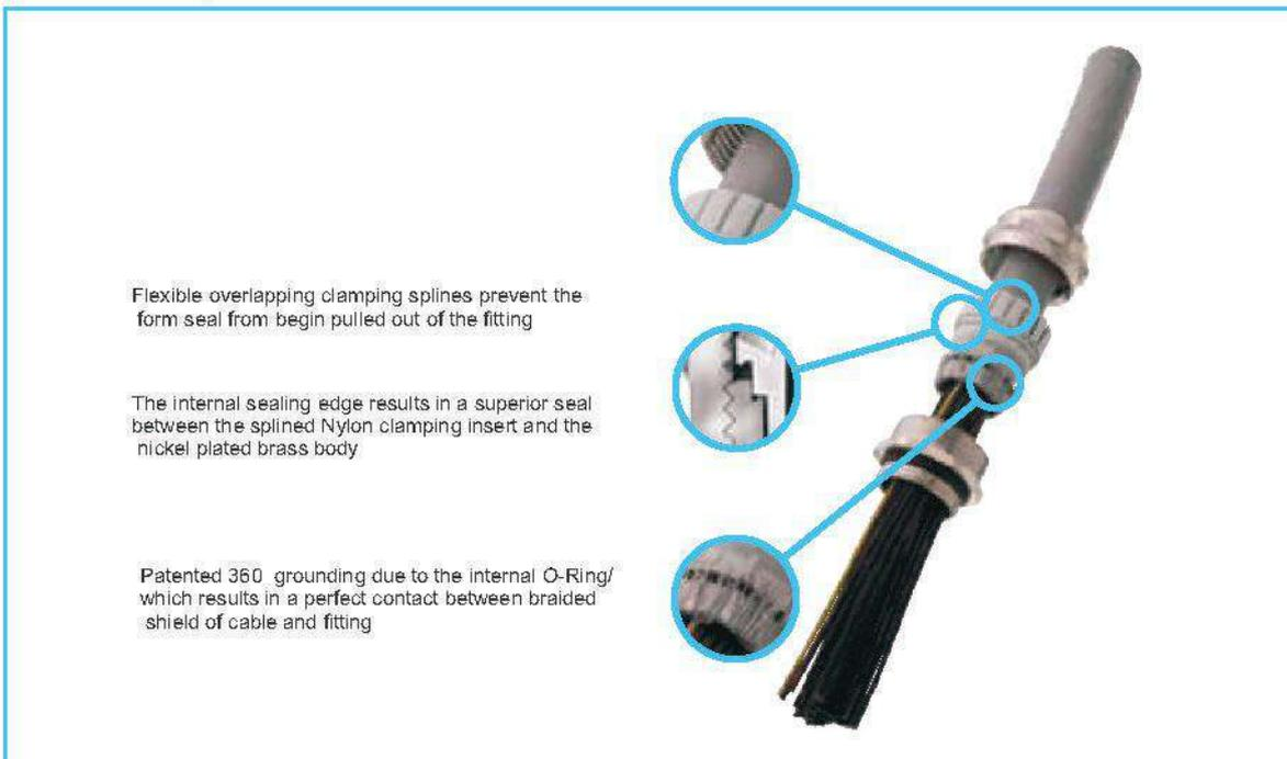
Flexible overlapping clamping splines prevent the form seal from being pulled out of the fitting
